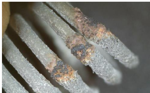
Fig. 14: 0.6 mm Kanthal AR wire after heating under the microscope. Note the reduction of the diameter of the wire as well as the spot where the wire oxidized and eventually failed.
