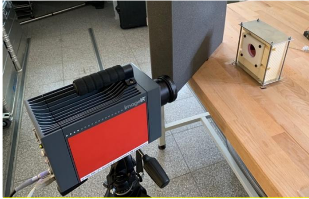
Fig. 22: Initial test setup with the IR camera and one thermally insulated lattice specimen filled with paraffin.
