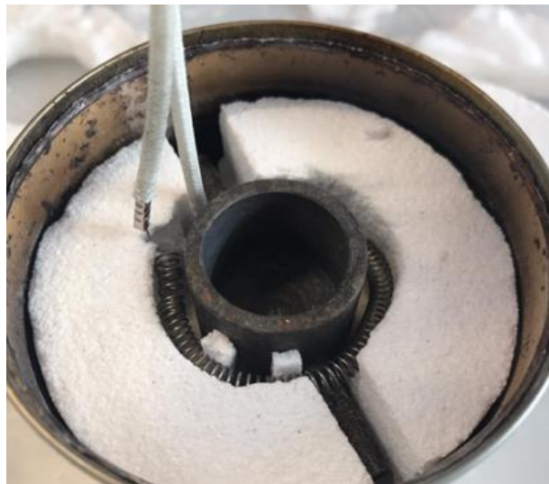
Fig. 11: The second prototype of a stainless-steel bushing embedded in UltraBoard® material surrounded by Kanthal AR heating wire
