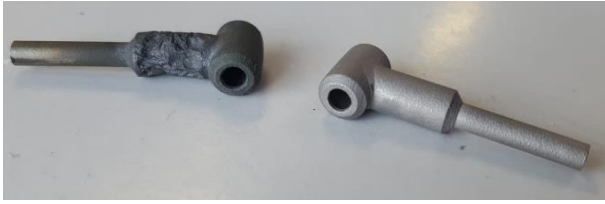
Fig. 26: Failed heated bushing (left) compared to a new one (right)
