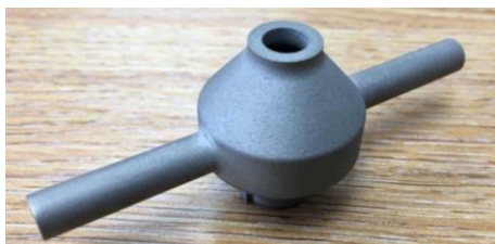
Fig. 8: PtRh bushing 3D-printed by Cooksongold
