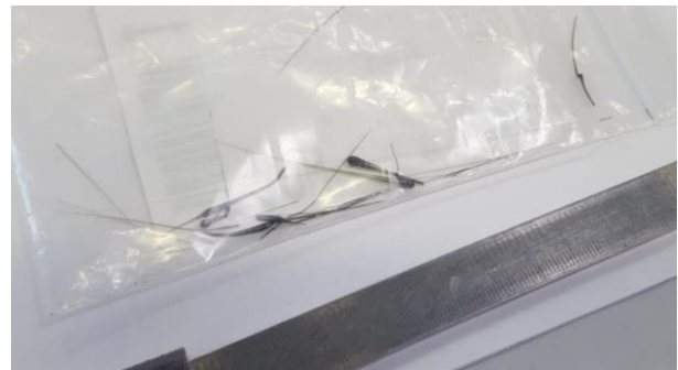
Fig. 18: Multiple E-glass fibers spun during the first spinning tests.
