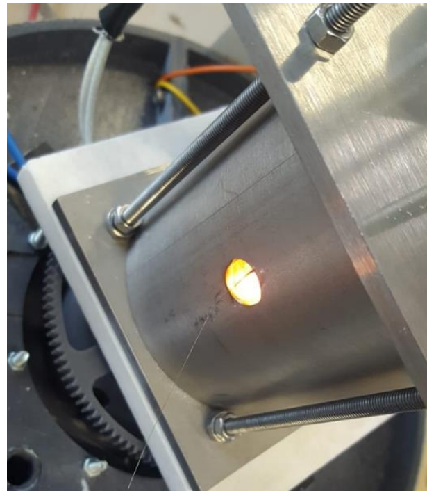
Fig. 17: E-glass fiber hanging for the bushing after the spinning test. Note the 3D-printed drive gear of the spinning apparatus and the white Teflon plate used to insulate it from the stainless-steel enclosure of the bushing assembly.
