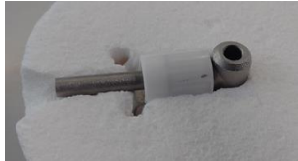
Fig. 24: 3D-printed stainless-steel bushing printed by EOS GmbH with the heating element. Note that the flight model of the bushing has two nozzles instead of one.
