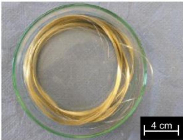
Figure 1. Macroscopic view of fibres made from ITALUS-2 [6]
