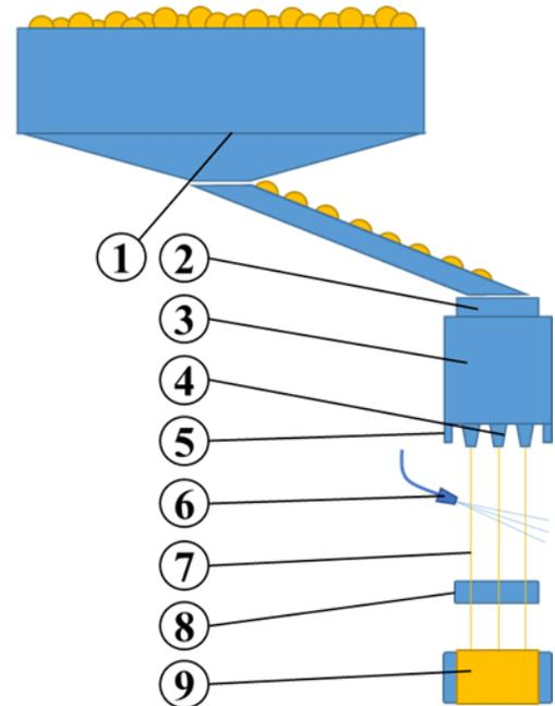
Figure 3. Terrestrial basalt fibre spinning process [5]; (1) – Raw material supply, (2) – Feeding & dosing system, (3) – Bushing, (4) – Nozzles, (5) – Cooling fins, (6) – Water spray for static discharging, (7) – Fibres, (8) – Sizing applicator, (9) – Winder
