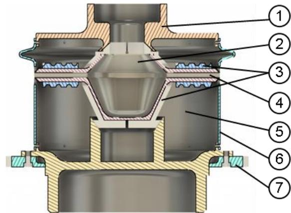
Figure 7. Bushing and its heating system and thermal isolation: (1) – Flange, (2) – PtRh Bushing, (3) – Ceramic Insulation for the heating wire, (4) – Nozzles, (5) – Wool insulation, (6) – Outer shell, (7) – Drivetrain gear
