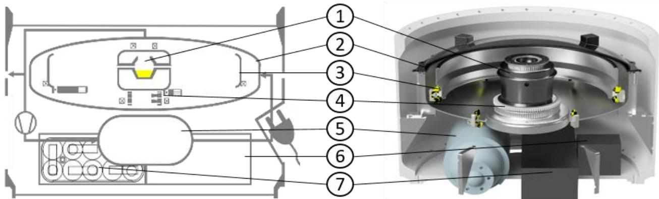
Figure 6. IMFEX Experiment concept: Schematic view (Left) and CAD Rendering (Right); (1) – Bushing, (2) – Pressure Vessel, (3) – Catching Drum, (4) – Bushing Drivetrain, (5) – Heat Exchanger, (6) – Computer Department, (7) – Battery Compartment
