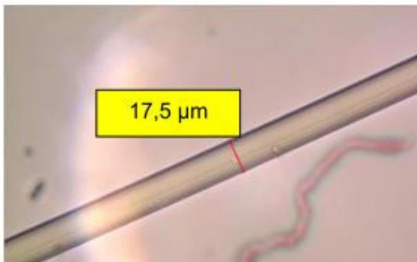
Figure 2. Microscopic view of fibres made from ITALUS-2 [6]
